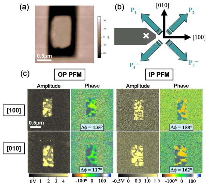
FIG. 2. (Color online) (a) Topography image of the BiFeO<sub>3</sub> nanostructure; (b) Schematic showing the cantilever alignment with the substrate orientation and the polarization directions of the BFO thin film, during PFM domain imaging. (c) IP and OP PFM images, obtained along the [100] and [010] directions.
