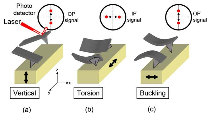
FIG. 1. (Color online) The three possible cantilever motions with respect to the orientation of the cantilever and polarization directions.
