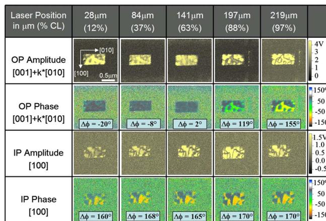
FIG. 3. (Color online) Montage of IP and OP PFM domain images taken along the BFO [010] direction with different laser spot positions along the length of AFM cantilever.
