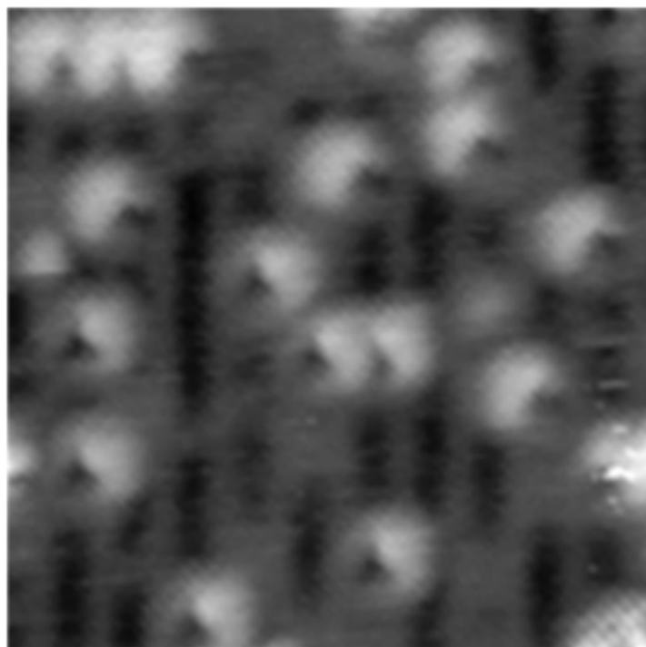
Figure 1.22 STM image exhibits strong trigonal intensity contrast, which implies the formation of (\text{WO}_3)_3 clusters on \text{TiO}_2(110) . This figure is reproduced from Ref. [126].
