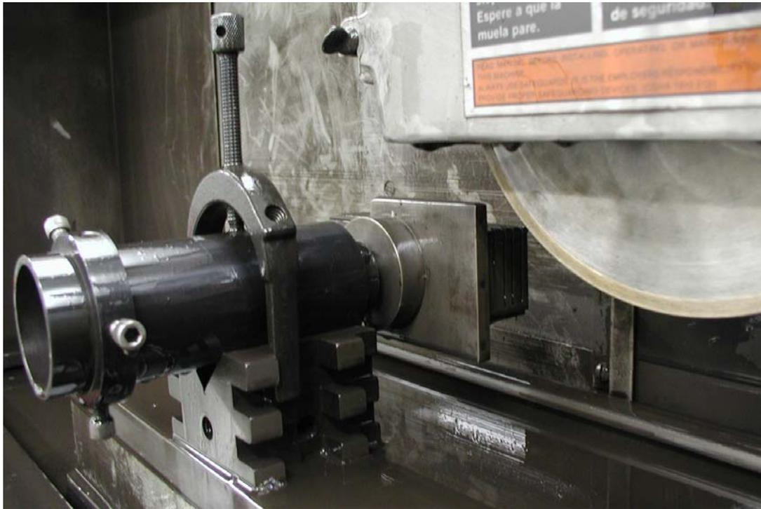
Figure B.8: Cutting the channel-cut monochromator with the diamond blade saw in the machine shop at DND-CAT. The Si block is mounted on the barrel-aligner and held with the V-block while the critical cuts are made with the saw. The external surfaces of Si crystal were bonded to 1/8" thick glass to prevent chipping and the cut was made in a single pass with an extremely slow transverse speed ( $\sim 0.1$  mm/s). The cutting fluid was shut off during this photograph.
